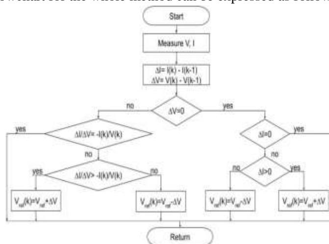
Fig. 5 Incremental Conductance Flowchart
