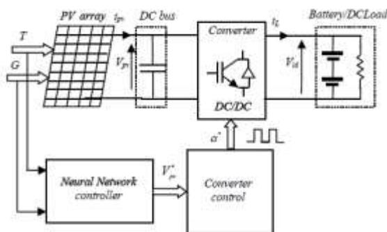
Fig. 1 Model scheme of the PV system
