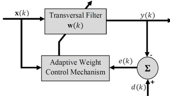
**Figure 2. Block Diagram of LMS Algorithm**
