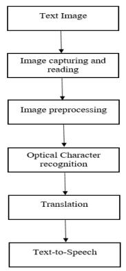
**Figure 3. Process flow**
