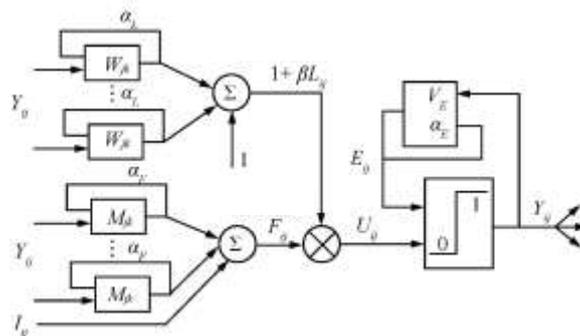
**Figure 1. A Typical Single PCNN Model**
