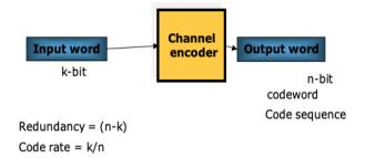
Fig 3: The channel encoders' block diagram
