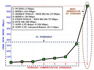
Fig 1: Ever increasing peak data rates of various wireless communication standards which include turbo code as their error.
