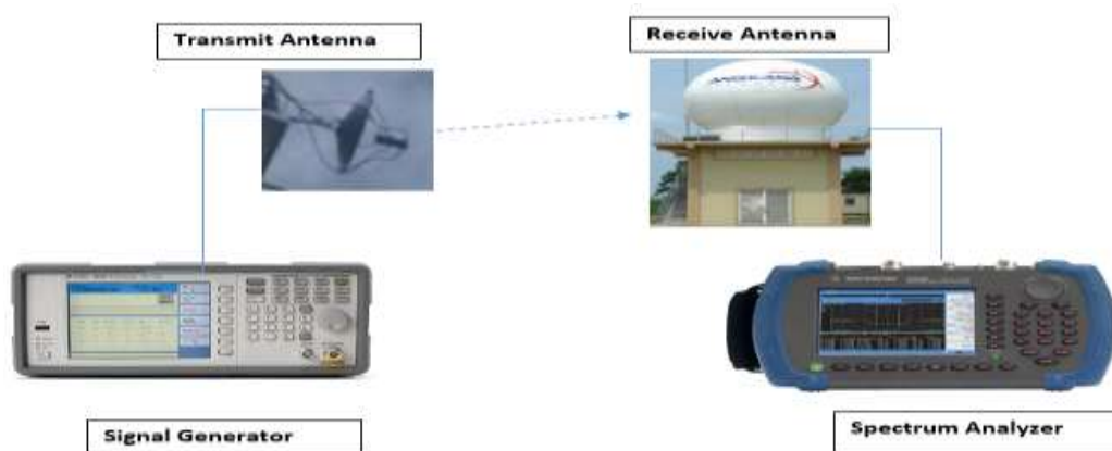
Figure 3. Setup for Power Received Measurement
