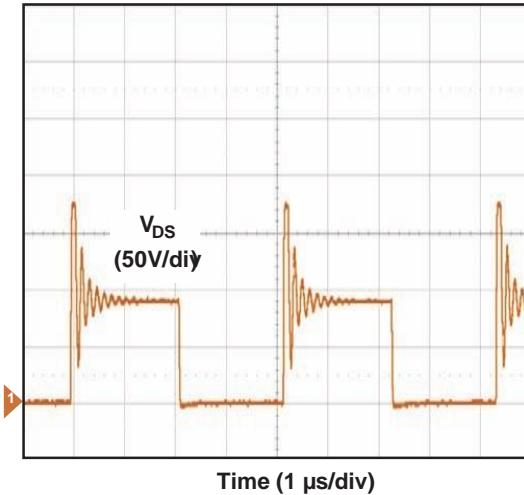
The active-clamp circuit, provides significant benefits versus an RCD clamp the drain-to-source voltage of the primary FET no longer has the large voltage spike when it is turned off. Instead of being dissipated in a resistor, the leakage energy is mostly recovered and returned to the input capacitors. Eliminating the leakage spike permits a primary FET with a lower VDS rating to be used, improving efficiency. Potential EMI issues are also significantly reduced.
