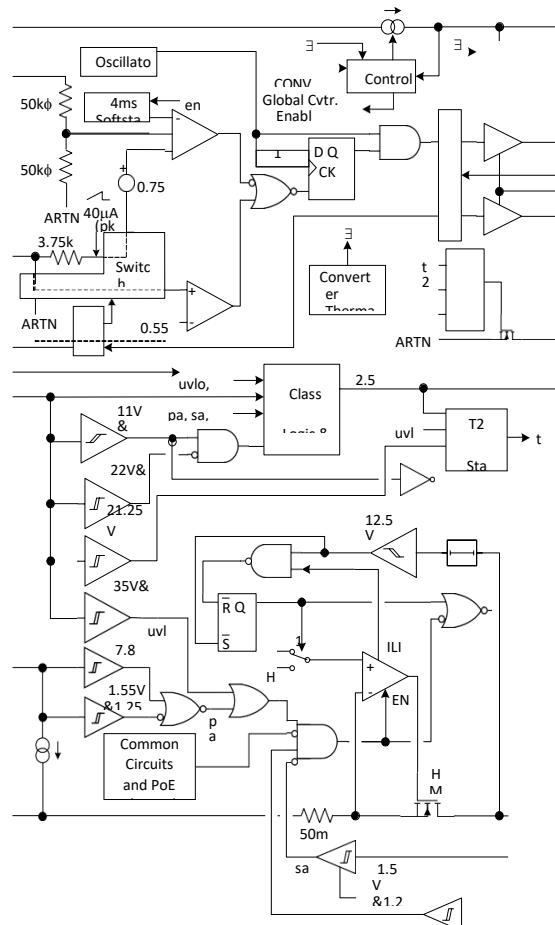
The Power over Ethernet interface attributes the new extended hardware classification necessary for compatibility with high-power midspan power sourcing equipment (PSE) per IEEE 802.3at. The detection signature pin may also be used to force power from the Power over Ethernet source off. Classification can be programmed to any of the outlined types with a single resistor.
