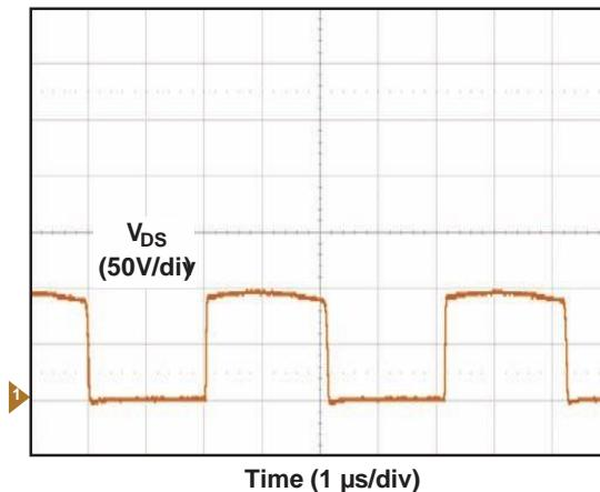
When Q1 is on, operation is the same as with a standard flyback converter. The current flows into the transformer's primary, storing energy in the primary's magnetizing and leakage inductances. During this time, Q2 and Q3 are off, while the output capacitor supplies current to the load.
