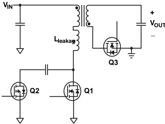
For a flyback converter operating in CCM, the transformer turns ratio and input-voltage range determine the duty-cycle range:
