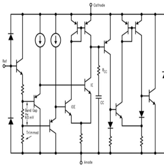
The LMV431, LMV431A and LMV431B have relatively initial tolerances of 1.5%, 1%, and 0.5%, and functionally lend themselves to several applications that prefer zener diode category performance at low voltages. Applications incorporate a 3 V to 2.7 V low drop-out regulator, an error amplifier in a 3 V off-line switching regulator and at the same time as a voltage detector. These parts are typically stable with capacitive loads greater than 10 nF and less than 50 pF.
