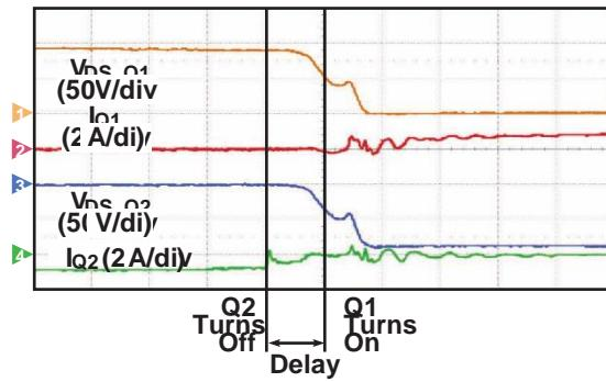
Assuming that the clamp frequency was properly chosen, the clamp current will flow from source to drain through Q2 before Q1 turns on. When Q2 is switched off, the clamp current will continue to flow through the body capacitance of Q2, resonating with the leakage inductance. The clamp current also commutes to the body capacitance of Q1, again resonating with the leakage inductance. It can be seen that Q2 switches off with 0 V across it.
