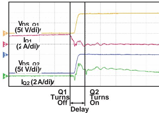
When Q1 is completely off, the current flowing in the leakage inductance is commuted from Q1 through the clamp capacitor and body diode of Q2 before Q2 actually turns on. After a delay time, Q2 is turned on with 0 V across it. The load and duty cycle have no effect, because the peak current is always flowing in the same direction during this transition.
