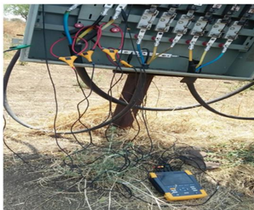
Fig. 2 Power analyzer connection on the LT side of Chandeale 3 DTR
