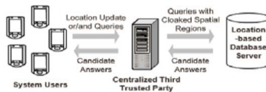
Figure 2: Casper Architecture – Variation of the centralized framework
