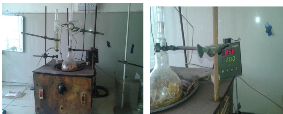
Fig 1. Oil bath with flask showing the liquefaction of bamboo
