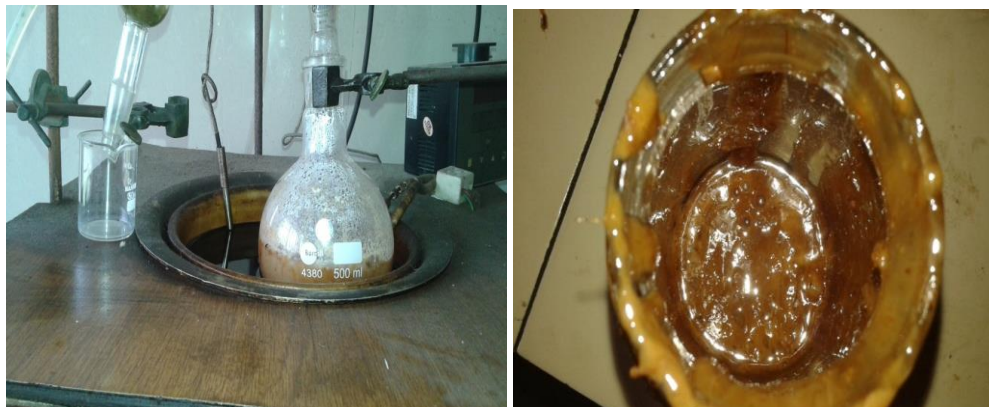
Fig 2. Oil bath with flask showing Adhesive mixture
