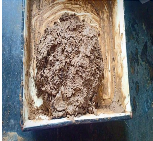
Figure 3. Reinforced Soil Sample with Human Hairs
