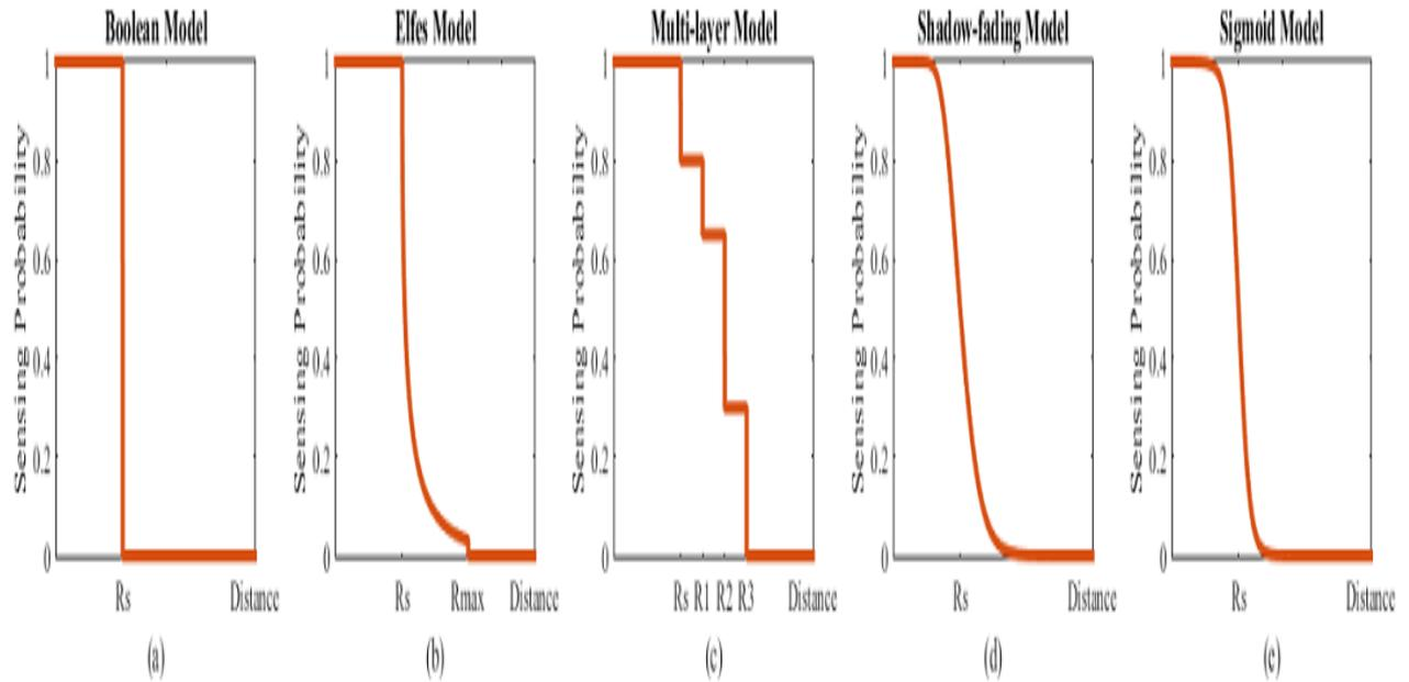
**Figure 1: Traditional sensing models. (a) Boolean model; (b) Elfes model; (c) multi-layer model; (d) shadow-fading model; (e) sigmoid model.**
