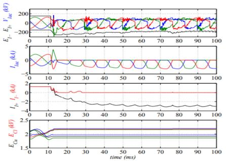
Figure 5.1 MMC station behavior when thyristor protections trigger 1.5 ms after the fault 5.2 Wind Power Plant power reduction during faults
