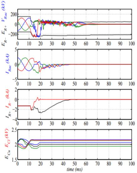
Figure 5.2 MMC station behavior when thyristors are triggered and wind power plant delivered power is reduced
