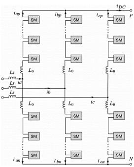
Figure 4.2. MMC topology where Ls is the phase input reactance, L0 is the arm reactance and SM is a submodule.
