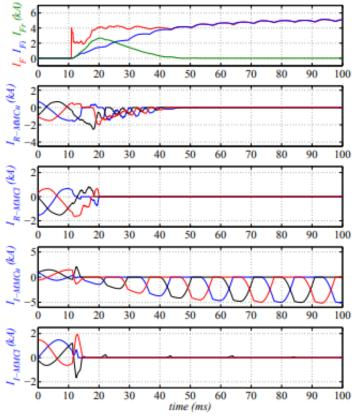
Figure 5.3 Fault and MMC branch currents when thyristors are triggered and WPP delivered power is reduced.
