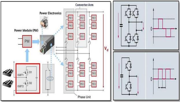
Figure 2.1 Modular Multilevel Converters
