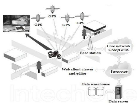
Fig. 2. The mobile monitoring system for pollutants control
