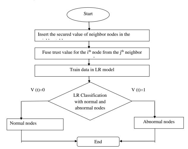
Fig 6: Flow chart for the logistic regression method detection of normal and abnormal packets
