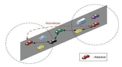
Fig 3: Wormhole attack on Manet https://www. 2Fnetworksimulationtools.com
