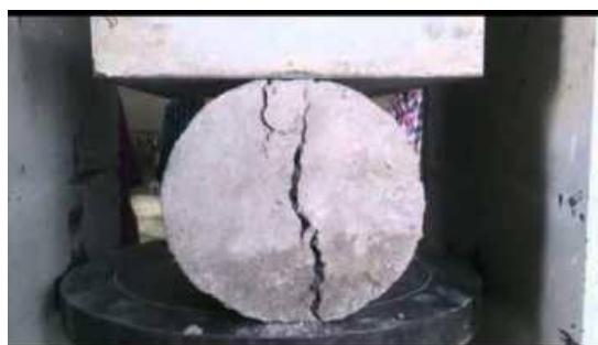
Figure 3:Split tensile strength of M30 Grade Concrete with different % of Recron 3S fiber and Sisal fiber after 7days, 14days and 28 days of curing.
