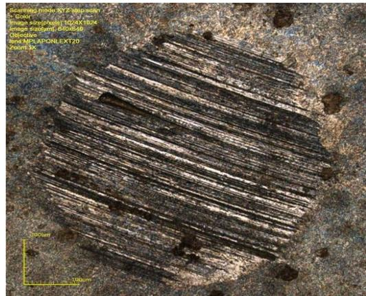
**Figure 6 image of wear topography obtained using confocal microscope .**
