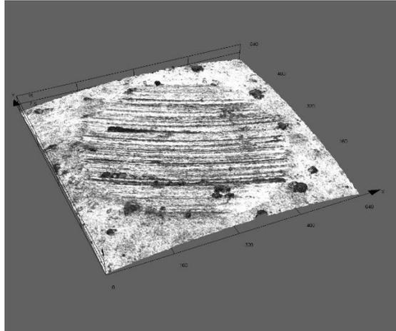
Figure 9. Image of wear topography obtained using a confocal microscope (0.8,0.2,0.8 wt.% Al<sub>2</sub>O<sub>3</sub>, SiO<sub>2</sub>, TiO<sub>2</sub>)
