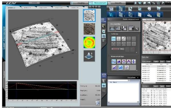
Figure 10. Image of wear topography obtained using a confocal microscope
