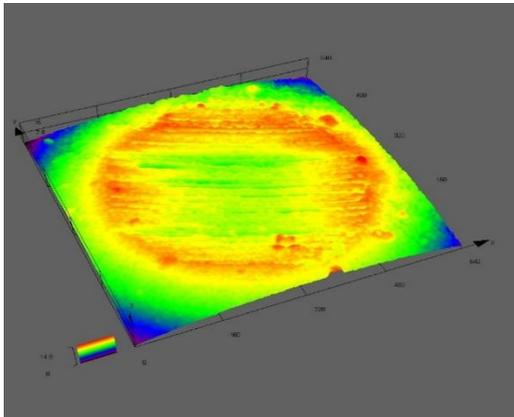
**Figure 5 image of wear topography obtained using confocal microscope**
