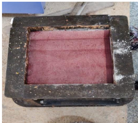
Figure 4 : Placing Geotextiles in top 1/5 th layer of non plastic soil layer.
