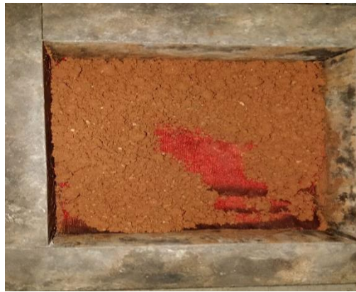
Figure 3 : Placing Geo textile in 1/5 th layer of soft soil layers
