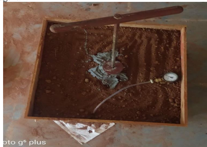
Figure 1: Grouting apparatus and wooden box
