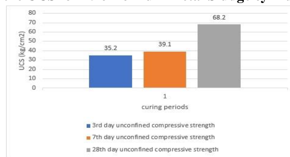
Figure 2: UCS curing trend for Chromium metal (Best Mix Design Batch as per UCS)
