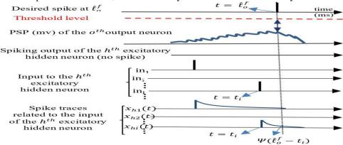
ISSN: 2233-7857 IJFGCN Copyright ©2020 SERSC Figure 1. Synaptic weight between *i*th input neuron and the *h*th excitatory hidden neuron  $w_{hi}$  is potentiated in proportion to the value of STDP time window  $[\psi(t-t_i)]$  at  $t = \hat{t}_o^f$  to generate hidden spike at the desired time  $t = \hat{t}_o^f$ . The generated excitatory input will be fed to the oth output neuron, and it increases the total PSP of the neuron at the desired time.
