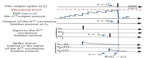
Figure 2.  $w_{hi}$ , the synaptic weight between *i*th input neuron and the *h*th excitatory hidden neuron, is reduced in proportion to  $\psi(t-t_i)$ , at  $t = \hat{t}_o^f$  (the time of the *f* th actual output spike of the *o*th output neuron). The reduction might lead to the cancelation of the hidden spike at  $t_h$  and consequently the reduction of the total PSP of the *o*th output neuron generated at  $t = \hat{t}_o^f$  and remove the actual output at  $t = \hat{t}_o^f$ .
