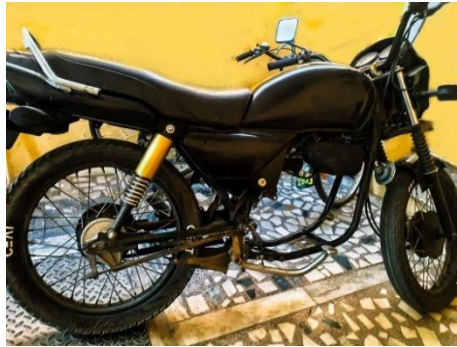
Fig.1 Frame of the vehicle without engine and gearbox
