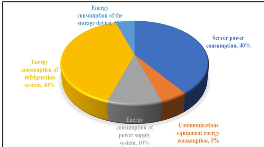
Figure 1 Energy consumption distribution of data centers
