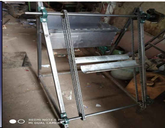
Fig.3.Actual drainage cleaner setup
