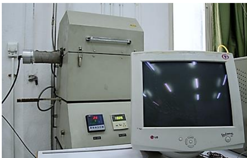
Figure 2b. Photographic View of TCVD Device
