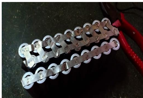
Fig.2 HCT Welded Spot
