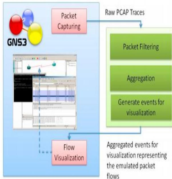
**Figure 5. Visualization of Packet Capturing and Analysis in GNS3.**
