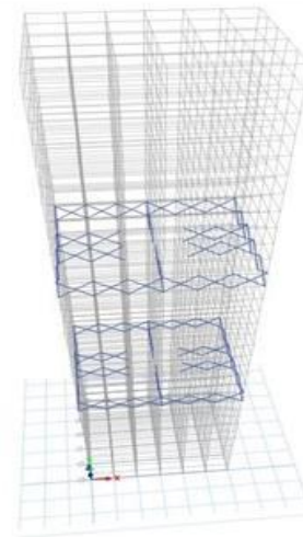
Fig. 4 3D Model with 2 Outriggers @ H/3 and 2H/3
