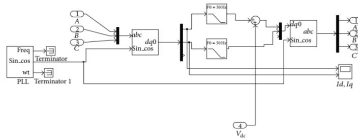
**Fig.3 Control topology for shunt filter**
