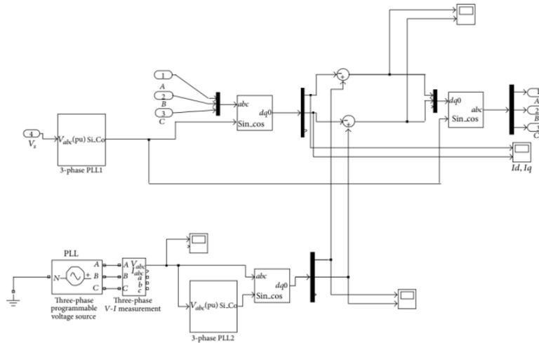
**Fig.2 Control topology for series converter**
