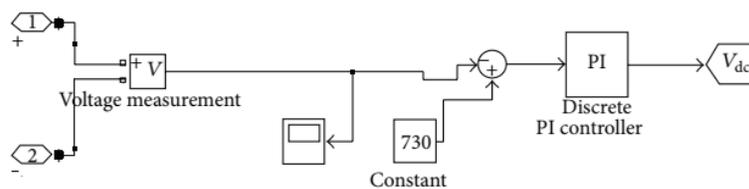
**Fig.4 Voltage at dc link**
