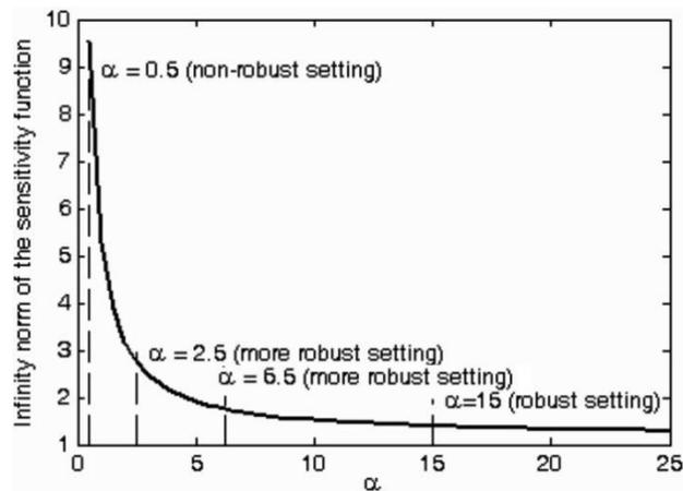
Fig. 4.  $H_\infty$  Standard of the sensitivity function with  $\alpha$
