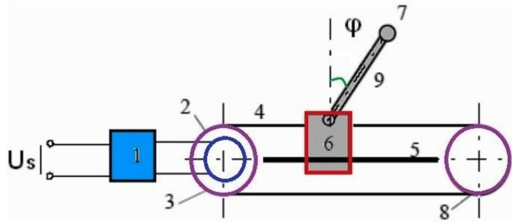
**Figure 1:** Design of Reversed pendulum
