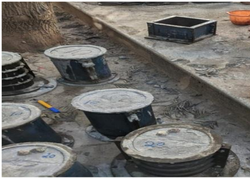
Figure 2.2 : Casting of cube specimen
