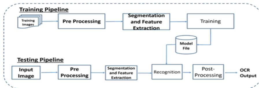
Fig. 1 Training & Testing flow.
