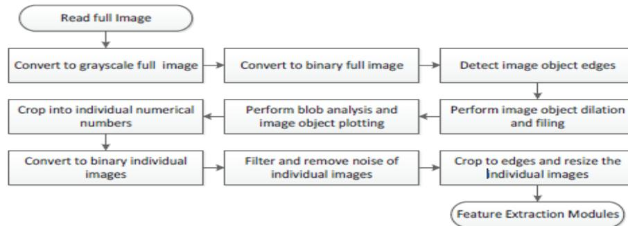
**Fig. 2** Raw Processing of Image before actual processing[11]
