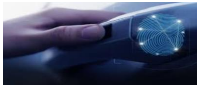
Fig.4 Car handle with fingerprint sensor.[8]
