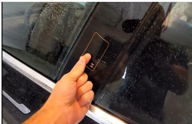
Fig.5 RFID chip read by RFID reader installed in car.
