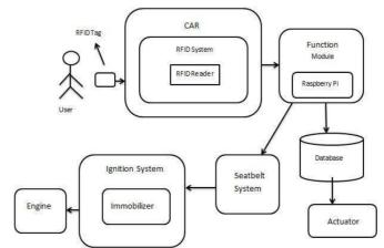
Fig. 1. Architecture of Security for Authentication & Security of user in car system.
