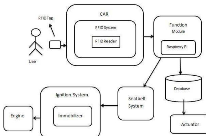
Fig. 1. Architecture of Security for Authentication & Security of user in car system.
