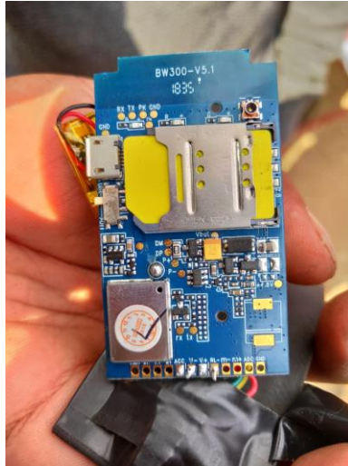
Fig. 3 The GSM module used to notify the owner incase of car theft.
