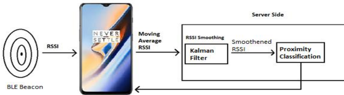
Figure 1: Working Principle of the BLE Beacon.
