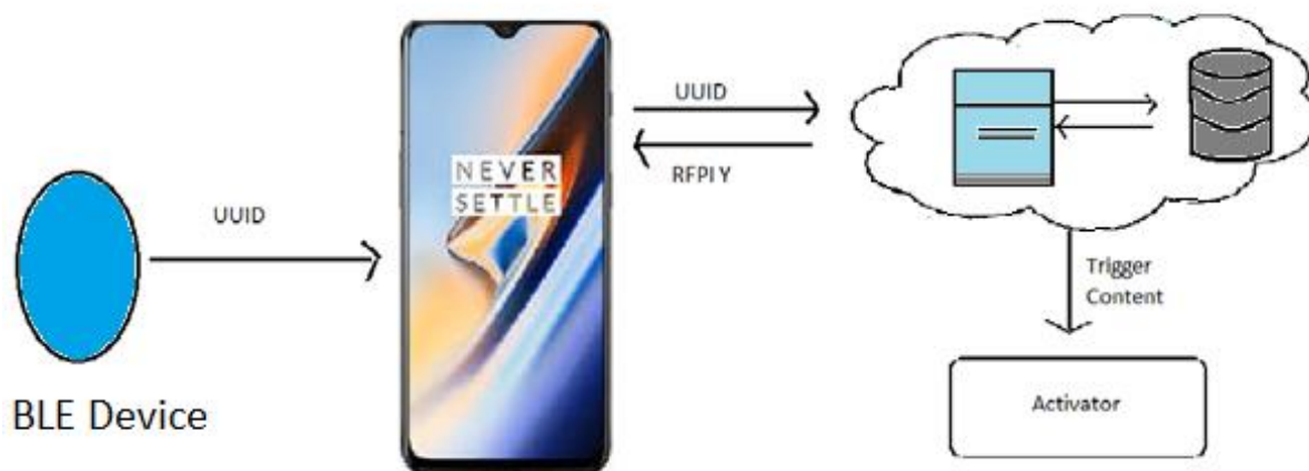
Figure 1: Working Principle of the BLE Beacon.
