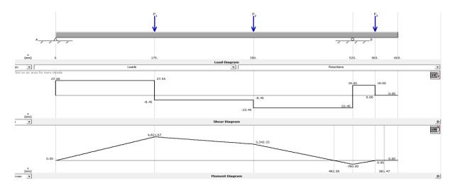
Figure 2: Schematic diagram showing SFD and BMD of vertical loading diagram of input shaft using MD Solid software
