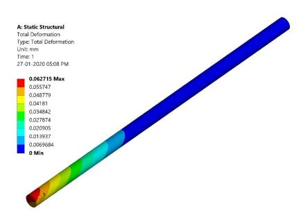
Figure 6: Total deformation of output shaft
