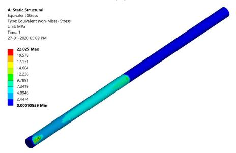
Figure 7: Equivalent Stress distribution on output shaft
