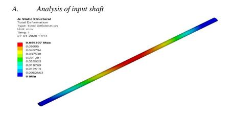
Figure 4: Total Deformation of input shaft
