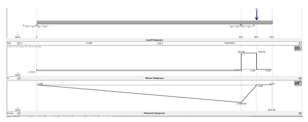
Figure 3: Schematic diagram showing SFD and BMD of horizontal loading diagram of input shaft using MD Solid software
