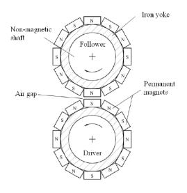
Figure 1: Parallel axis magnetic gears [3]
