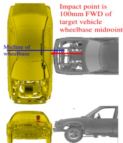
Figure 1: Side Impact Configuration
