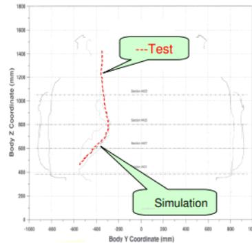
Figure 5: Intrusion Comparison
