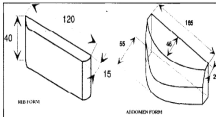
Figure 8: Dimension used for foam
