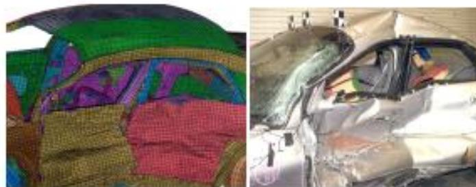
Figure 2: Deformation in model with curtain airbags
