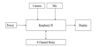
The given block diagram shows the basic architecture of the proposed smart speculum.:
