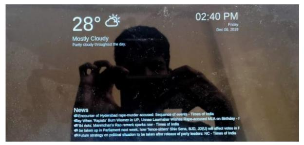
The following image shows the output of the smart speculum. It has shows the current system time, the weather information and the news headlines of the day.
