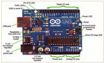
Figure.3.1 Arduino Board
