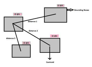
Figure 2. Distance Detection Algorithm using Centroid as Reference
