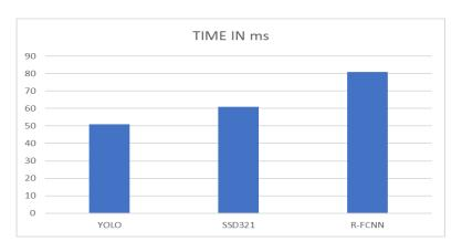
Figure 4. Graphical analysis of Time of different algorithm
