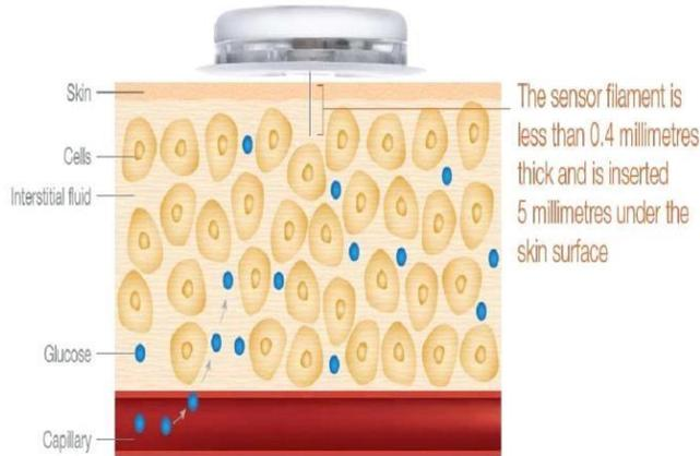
Fig.6 Interstitial fluid (ISF) Based Glucose sensor
