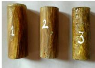
Figure 3: Compression Test Specimen
