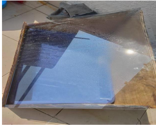
Fig.4 Single effect, single slope/basin type passive solar still system
