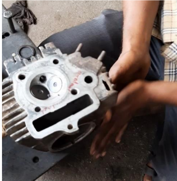
Fig 4:Hand Valve Lapping Process
