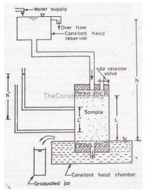
Fig.2: Constant Head Permeability Test
