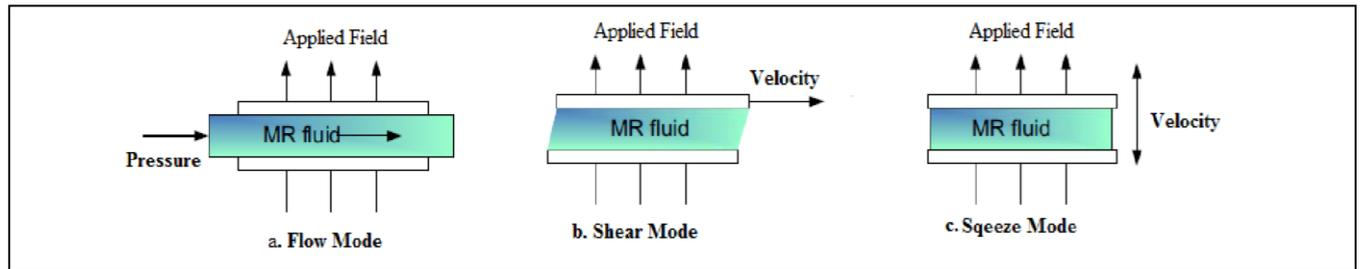
Fig. 2: Modes of Operation of MR Damper
