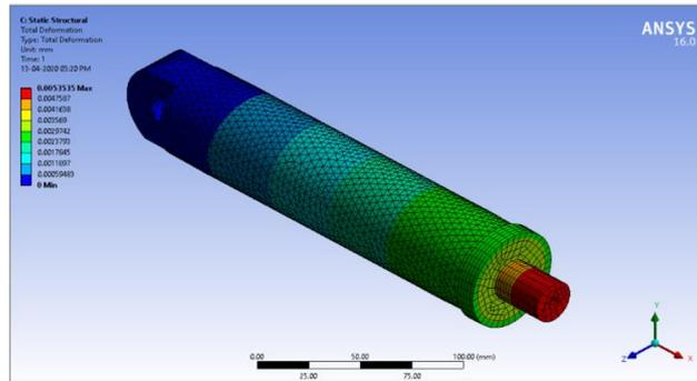
Fig.7: Total Deformation of Damper
