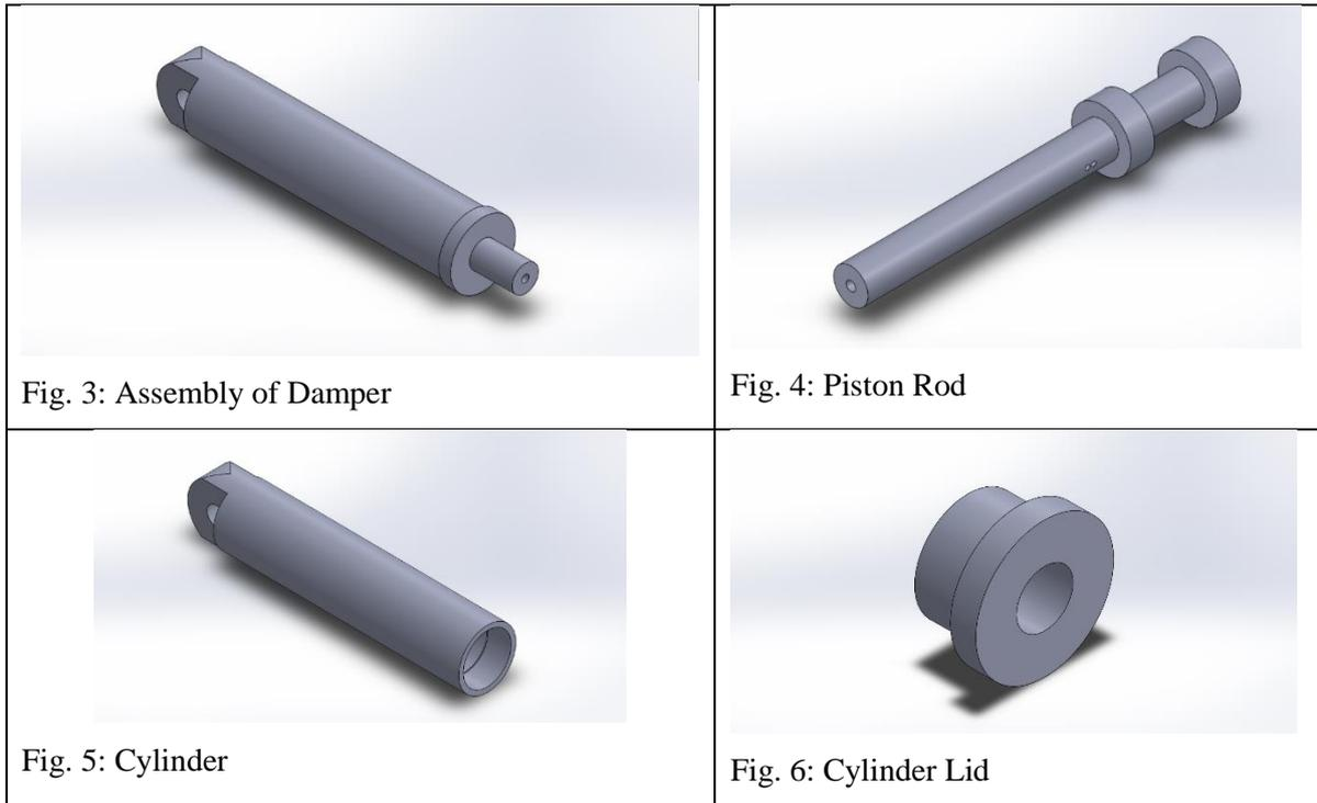
Piston of MR Damper is wrapped into a magnetic coil. Holes are provided to pass the coil inside the cylinder. The function of piston in conventional damper and MR damper is same i.e. to force the fluid through valves or annular space. As shown in fig 4, a groove is provided on piston surface for coil. The required dimensions of groove were designed. The single tube cylinder as shown in fig 3.3 is used in this work. A lid (shown in figure 3.4) is provided to prevent the flow of liquid out.
