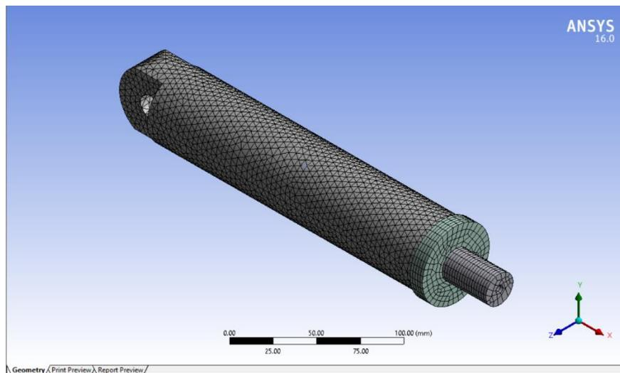
Fig.7: Meshing model of Damper
