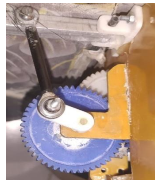
Fig. 6 Assembly flapping mechanism
