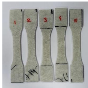
Fig. 5 Glass Fibre Specimens after testing
