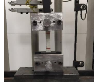
Fig. 6 Flax after testing
