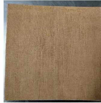
Fig. 2 Flax Polyester Composite Laminate
